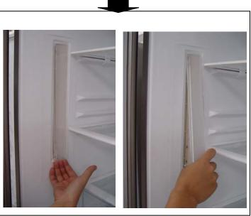
Step3. Remove LED pcb board and then disconnec the terminal.
