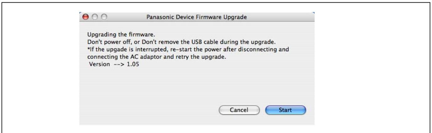
8. The following window is displayed during software update. Don't disconnect the USB cable or turn off the power during software update. Update time is approximately 10 minutes.
