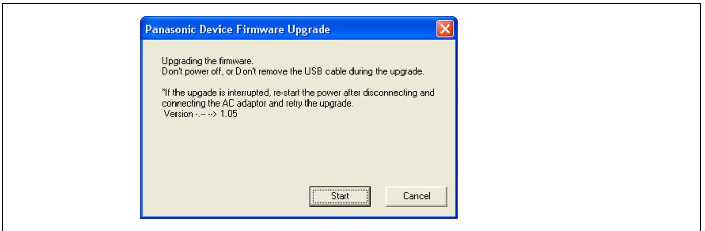
9. The following window is displayed during software update. Don't disconnect the USB cable or turn off the power during software update. Update time is approximately 10 minutes.
