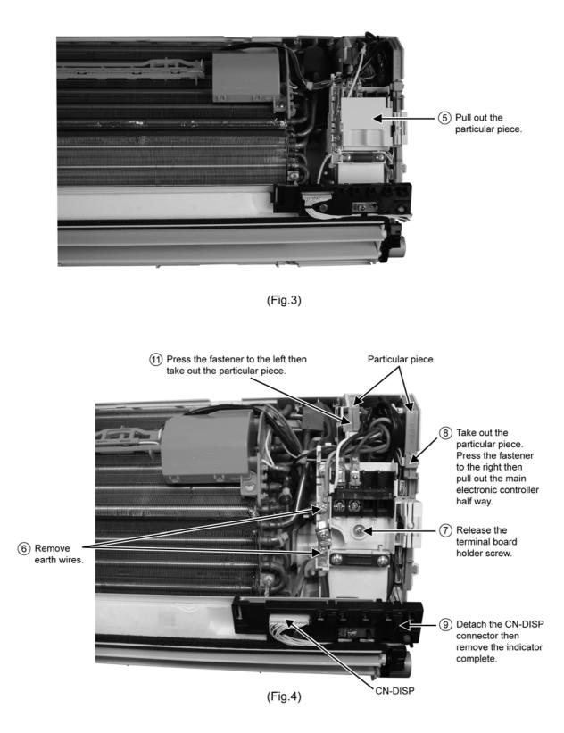
(1) Detach 5 connectors as labeled from the electronic controller. Then pull out slowly while pressing the fastener to the right.
